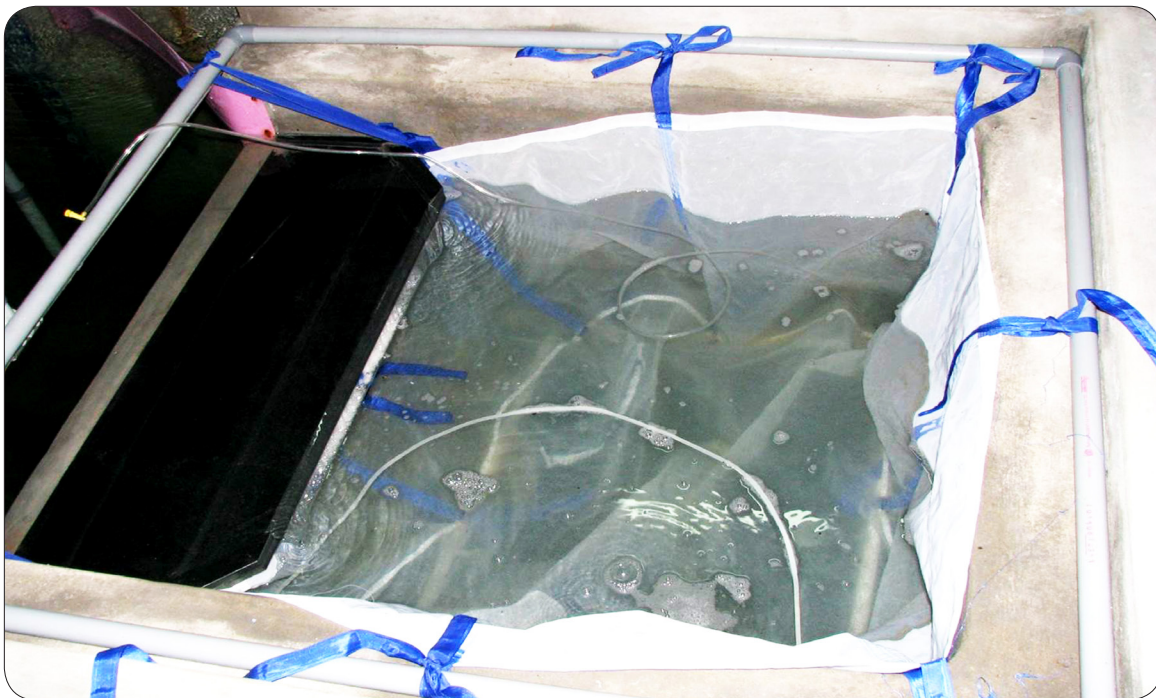
Automatic egg collection device in spawning tank
